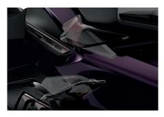
ADJUSTABLE SIDE WIND DEFLECTORS Regulate driver and passenger lower-body airflow. Change to closed, open or parallel position for optimal comfort. Simple, tool-free adjustment so you can spend more time riding.
